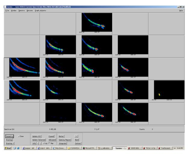
Calibration of CsI with recoil protons from <sup>40</sup>Ca + CH<sub>2</sub> reaction
