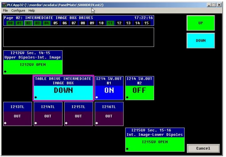
On page 2 of the S800 drives page: The "table drive intermediate image box" can be used to insert and retract the tracking PPACs.
