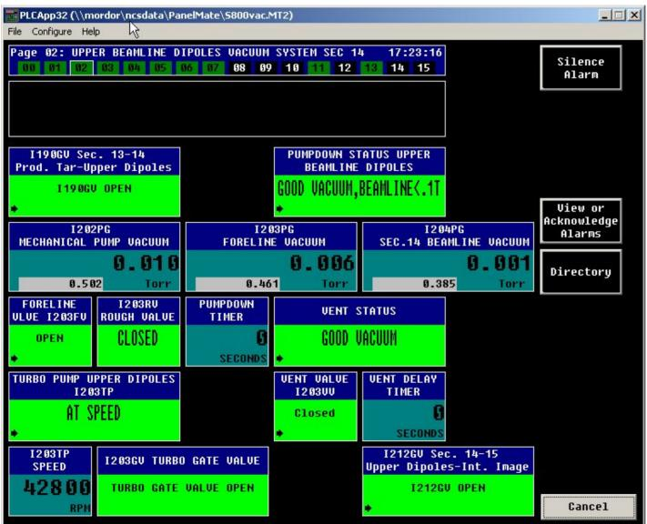
Displays the status of the vacuum from the S800 object ("production target box") page 1 to the focal plane on page 7. All gate valves can be controlled from there. Important gate valves for experimenters:
