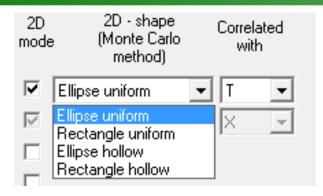
Four 2D-shapes. Hollow configurations (which are not physical) are designed for debug purposes
