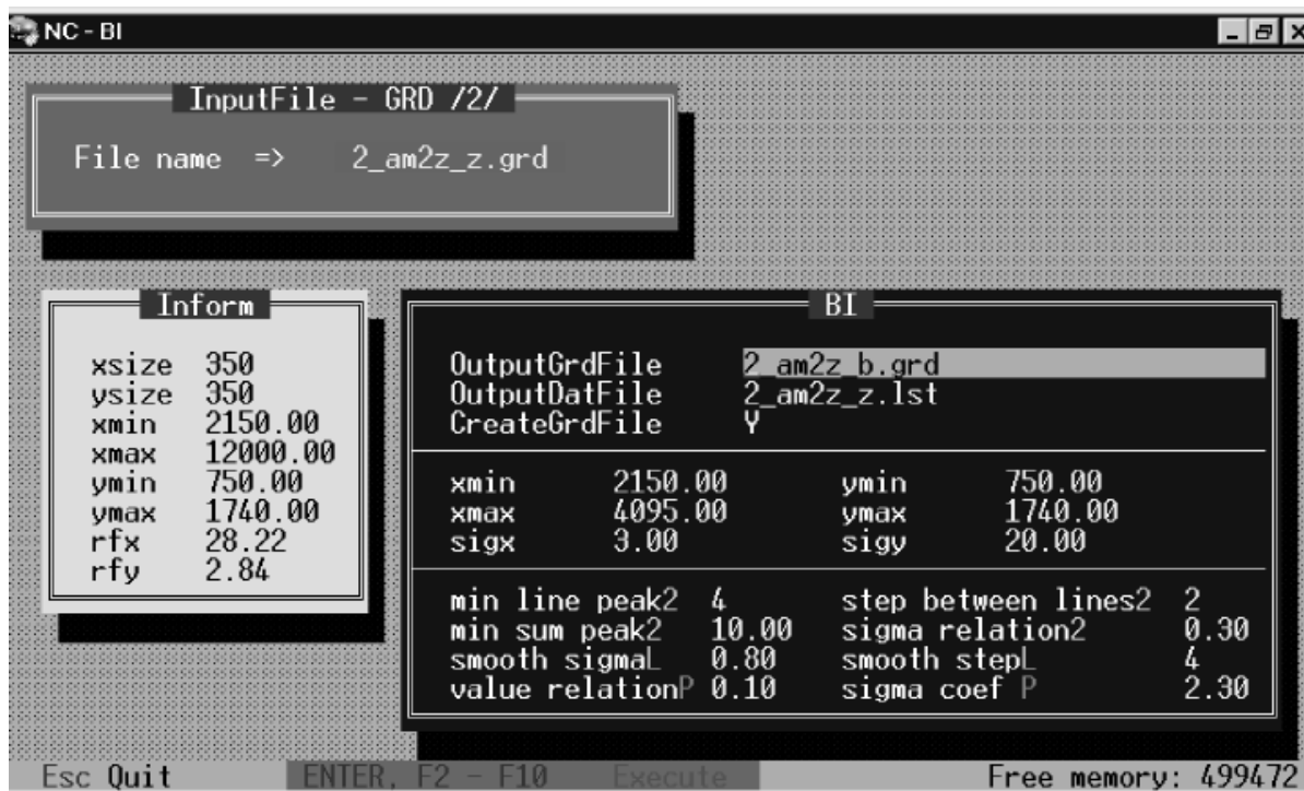
Fig.1. Principal window of the code “BI” (version for MS-DOS) designed for automatic search of two-dimensional peaks and definition of their characteristics.
