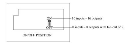
At power on, the green LED "M" lights up if the module is set to the single input-single output configuration.
