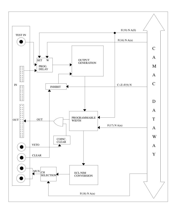
Figure 1 Block Diagram of the Mod. C 469
