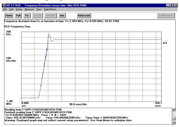
This is a display of frequency deviation from a constant reference frequency, Fo. The reference shows up in the display as a green line at a value of zero. The Fo computed by the software is displayed in the log at the bottom of the display. This value can be recalled at any time, along with the pacing value and the total number of samples by clicking the **Fo** button on the tool bar.
