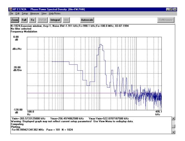
This display was computed from the "fm.pan" data. This is the power spectral density plot of the modulating tone. The 11 kHz modulation is easily seen on this display, as well as other modulation products.
