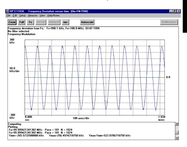
"Frequency deviation from Fo as function of time. Fs=9.901 kHz; Fo=100 MHz; 03/07/1994"
