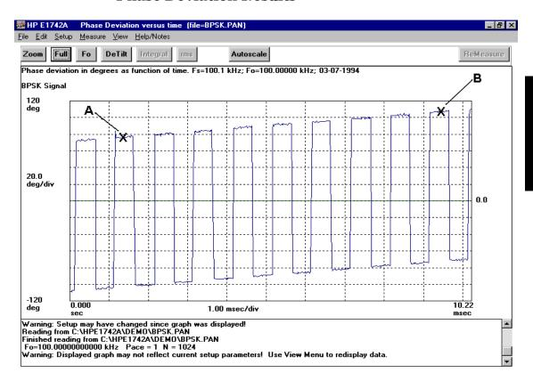
This is a display of phase deviation from the constant reference frequency,  $Fo = 100 \ \text{kHz}$ . The square wave modulation can easily be seen. Using the cursor (left mouse button) and delta cursor (right mouse button) features, you can easily determine the period of the modulation (1/mod rate), and the peak-to-peak values.
