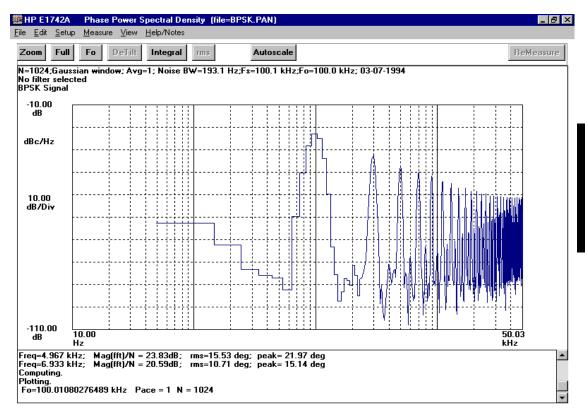
This plot is very similar to the FFT. Since it is normalized, the units are in dBc/Hz. Note that the top line of the display shows the noise bandwidth.
