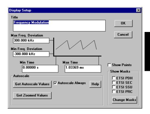
The Display Setup menu lets you annotate the display with a title, date, or other descriptive information which may be useful if you store the data to a file or print a hard copy. You can also set the scaling for both the x and y axis of the measurement display or select the  $\bf Autoscale$  function. Display masks can also be turned on in the Display Setup dialog box. Search the HP E1742A/46A/48A on-line Help for  $\bf Show\ Masks$  to obtain more information.
