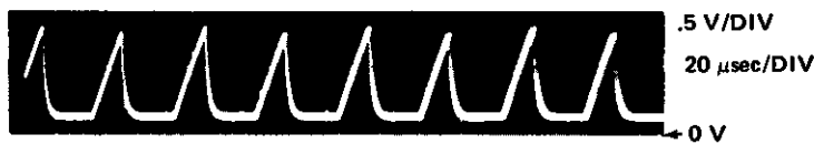
J.) At TP1919. Mono Ramp during normal operation.
