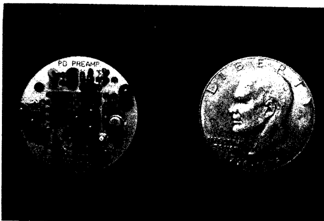
Fig. 1: Photograph of the Photo Diode preamplifier. Notice the small size, even though standard Semiconductor packages were used.
