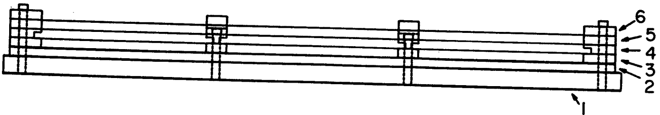
Fig. 2. Cross-sectional view of one APEX detector element. 1) 1/4" thick aluminum or magnesium back plate, 2) 1/64" thick meander PC board, 3) anode plane, 4) front cathode plane, 5) pressure window frame, 6) support wire frame.
