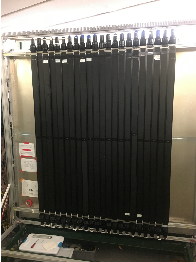
Figure 2.20 A picture of the Veto wall (VW). The VW consists of 25 vertical plastic scintillator bars. PMTs are installed at both ends of each bar. Photo courtesy of K. Zhu.
