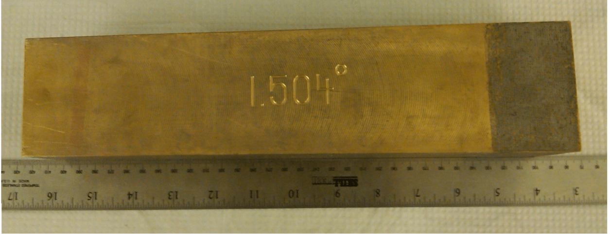
Figure 3.17: A shadow bar used in experiments for background neutron scattering efficiency correction. Picture is adopted from Ref. [15].
