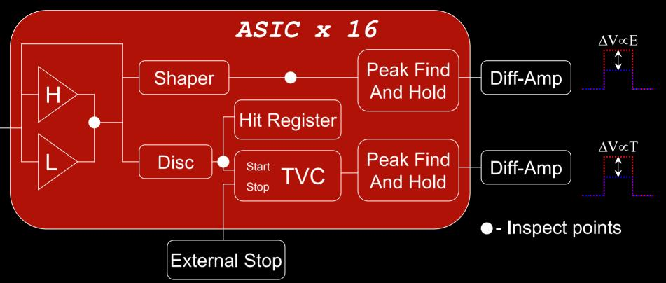
✓ 2 different gain internal Charge Sensitive Amplifiers (CSA)
