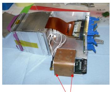
Step3: Removing these two screws will allow to take out PA box from the telescope. To get access of the preamps, you need to uncover the copper plate.
