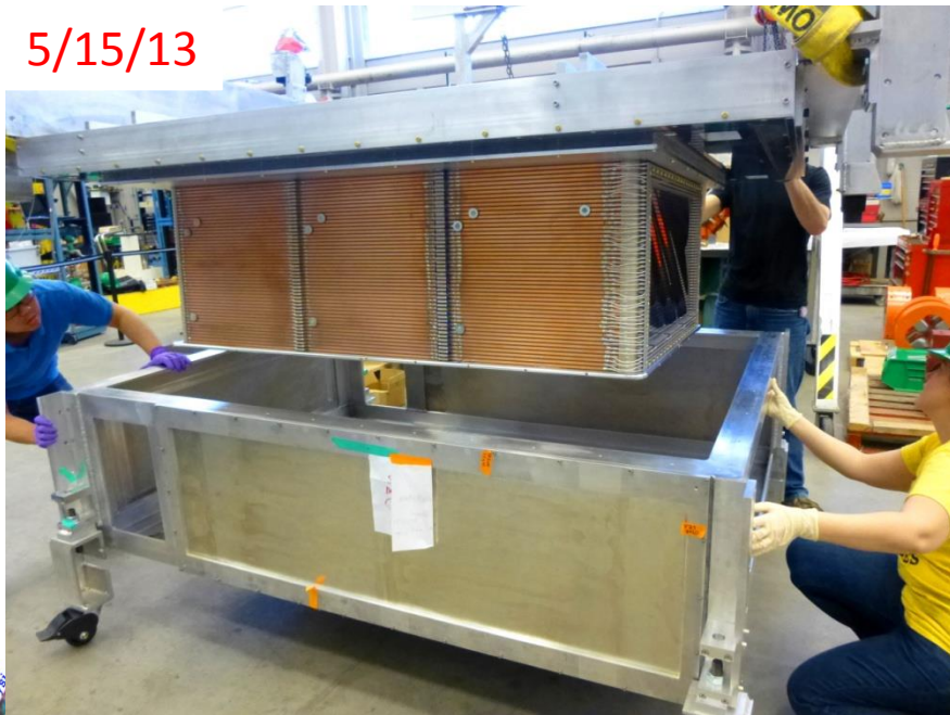
Installation of Field Cage
