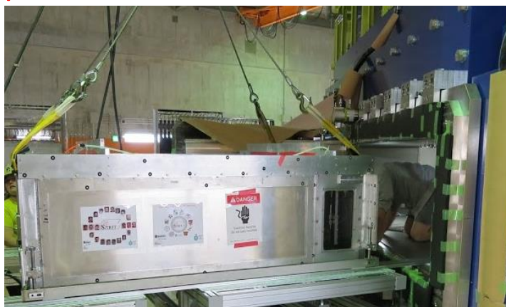
\pi RIT TPC inserted inside the SAMURAI Magnet Chamber 7/23/2014
