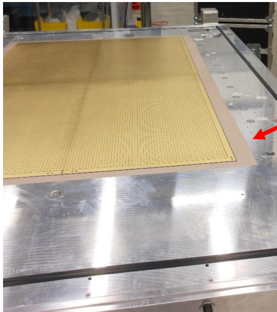
Pad plane is attached to large aluminum plate
