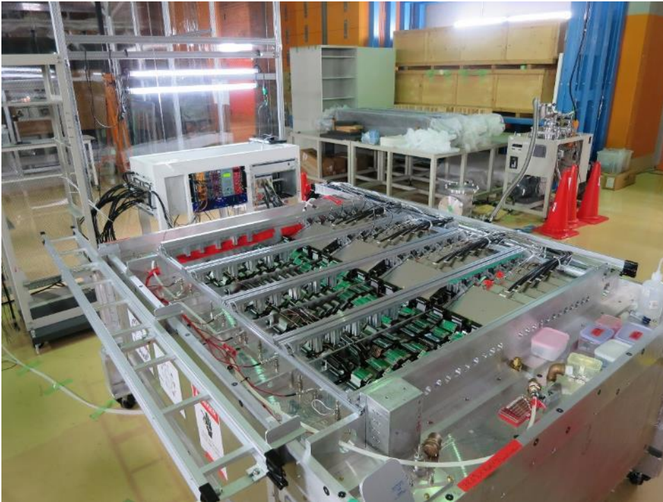
TPC with GET electronics installed on half of pad plane
