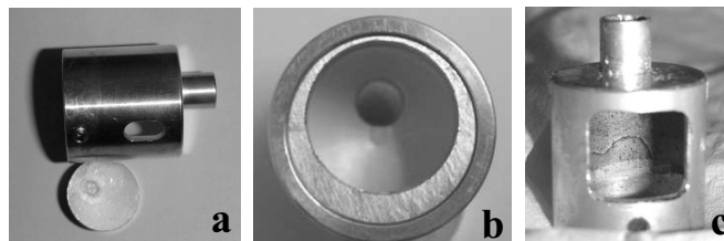
Figure 4.14: Photographs of (a) an ablated Ag target with Holder B, (b) the added collar to hold the Ag and Zn targets (no target present), and (c) the opening of Holder B that was modified to make it larger for more of the plume to escape.
