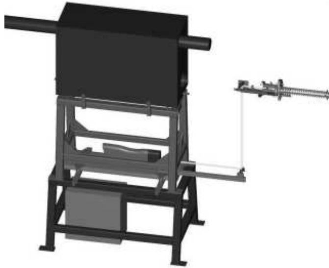
Figure 4.7: A CAD view of the laser ablation system. The laser head rests on an optical table mounted under the last superconducting magnet on the heavy-ion beamline to the gas cell. The entire laser system is enclosed in a safety enclosure to contain any stray light.
