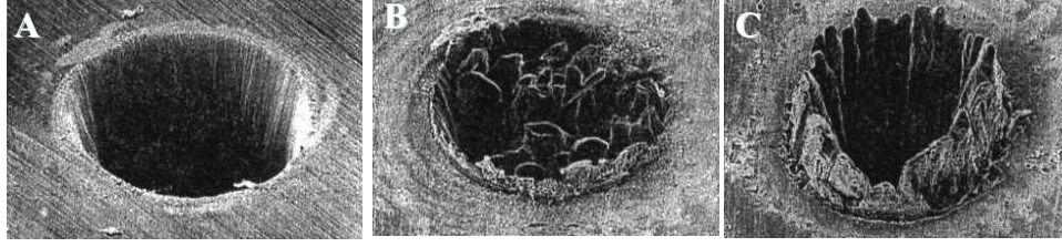
Figure 2.2: A comparison of the laser-induced craters for three different pulse lengths: (A) 200 fs (B) 80 ps and (C) 3.3 ns, from [31]. As the pulse length increases, there is more interaction between the material and the laser pulse. In addition, there is matter in both liquid and vapor form for ns ablation.
