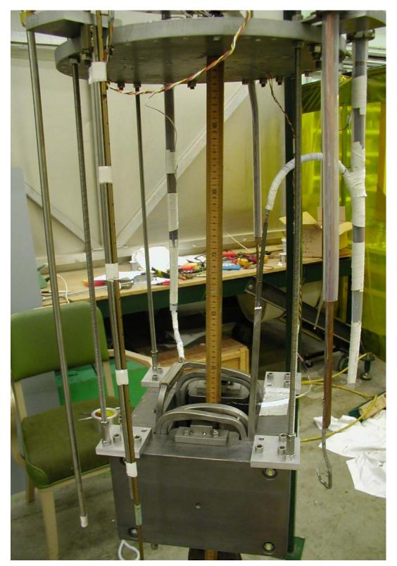
Fig. 3-9: The MOCICC dipole hangs under the NSCL dunking Dewar lid, ready to be tested. The magnet leads have been connected to the Dewar leads.
