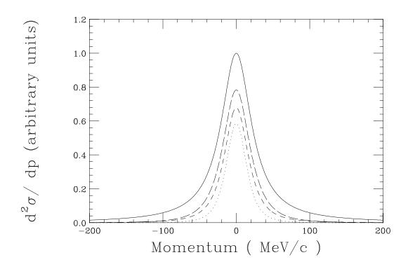
Figure E.1: The expected  $p_{\parallel}$  distributions for a fragment with  $p_{ave}=3400 \text{ MeV/c}$ and with  $\Gamma=50 \text{ MeV/c}$  are shown for complete acceptance (solid), for an acceptance similar to that of the A1200 Spectrograph medium acceptance mode (long dashes), for a pinhole acceptance (short dashes X10), and for a horizontal line acceptance (dots X100). See Table 1 for details.
