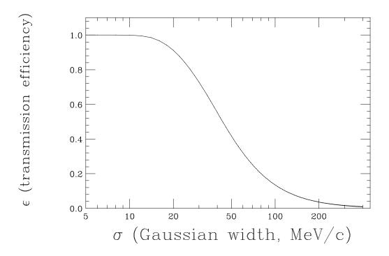
Figure E.3: The transmission of the A1200 spectrograph for a Gaussian distribution as a function of its standard deviation. The curve is calculated for <sup>10</sup>Be fragments with  $p_{ave}=3400 \text{ MeV/c}$  produced in the A1200 medium acceptance mode, ( $\Delta \theta = \pm 20$ mrad and  $\Delta \phi = \pm 10$  mrad).
