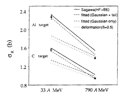
Figure B.2: [Fuk91] The energy dependence of the <sup>11</sup>Be reaction cross section. The two models that fit the trend of the data both include a large halo, while a deformation in <sup>11</sup>Be does not reproduce the data.
