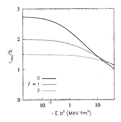
Figure A.2: [Rii92] The dependence of the rms radius of a valence proton on binding energy for a nucleus that has four protons in the core, for example  ${}^{8}B$ .
