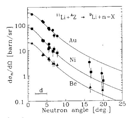
Figure 2.2: [Ann90] The angular distribution of neutrons following the breakup of <sup>11</sup>Li are compared with Lorentzian shapes. The deduced widths are small,  $24\pm4$  MeV/c FWHM.
