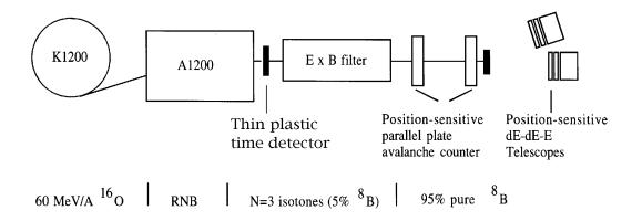
Figure 4.3: A schematic illustration showing the overall layout of experimental apparatus used in the <sup>8</sup>B breakup experiment.
