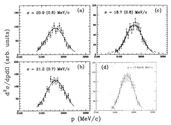
Figure 2.4: [Orr92] and [Orr95] The  $p_{\parallel}$  distribution of <sup>9</sup>Li fragments following the breakup of 66A MeV <sup>11</sup>Li in <sup>9</sup>Be, <sup>93</sup>Nb, <sup>181</sup>Ta and <sup>238</sup>U targets, (a) through (d) respectively. In (c) the dashed line is a dipole excitation calculation, Section 2.3.3, that is in excellent agreement with the data.
