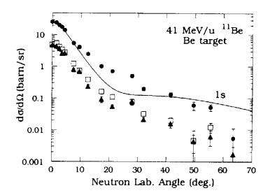
Figure 3.18: [Ann94] The angular distribution of neutrons following the beakup of 41A MeV <sup>11</sup>Be is in agreement with a prediction based on a 2s-orbital neutron (1s in some notation) in a simple square-well potential. A narrow width ( $\Gamma$ =60 MeV/c) is extracted from the restricted inclusive data ( circles, n+ no <sup>10</sup>Be). Also shown are the distributions for n+He (triangles) and n+Li (squares).
