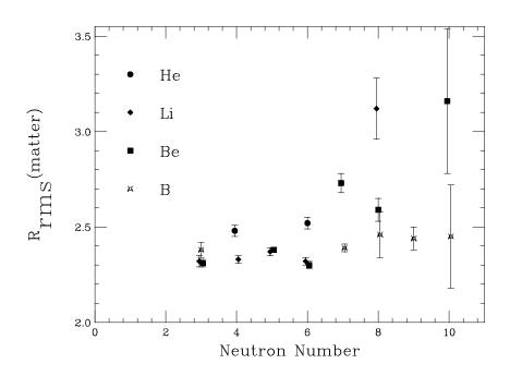
Figure 1.1: The rms radii obtained from the 790A MeV cross section measurements. The nuclei <sup>6</sup>He, <sup>8</sup>He, <sup>11</sup>Be, <sup>14</sup>Be and <sup>11</sup>Li are noticeably larger than other nuclei in this region. Data from [Tan88].
