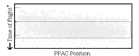
Figure 3.8: The most selective condition is on the Time of Flight<sup>\*</sup> vs. X focal plane position histogram. Time of Flight<sup>\*</sup> is a pseudo-parameter, based on the real Time of Flight, that removes the position dependence of the Time of Flight for particles that have different path lengths through the dipoles (related to different radii of curvature).
