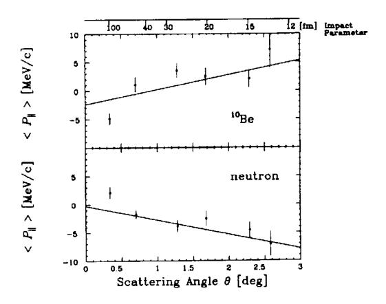
Figure B.4: [Nak94] The mean momentum of breakup neutrons and <sup>10</sup>Be cores plotted vs. the center of mass angle. The trend expected from Coulomb reacceleration is observed. This strongly favors a direct breakup interpretation of the data from <sup>11</sup>Be Coulomb breakup.
