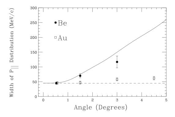
Figure E.2: The expected  $p_{\parallel}$  distribution from a Lorentzian density distribution (solid) and a Gaussian density distribution (dashed) compared with data from the breakup of <sup>11</sup>Li in the S320 [She95]. For this case  $p_{\perp}=p_{ave}\sin(\theta)$  where  $p_{ave}=2300$  MeV/c. Details are given in the text.
