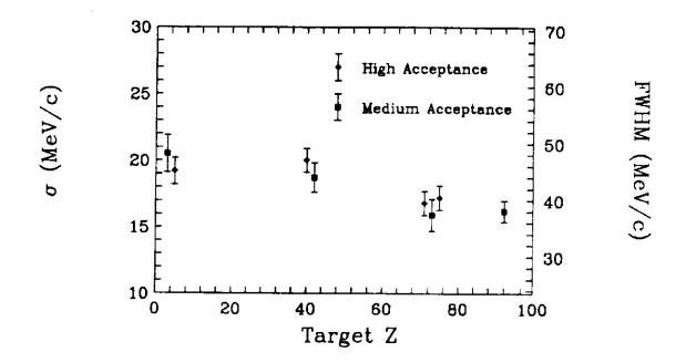
Figure 2.5: [Orr95] The  $p_{\parallel}$  distribution widths of <sup>9</sup>Li fragments from <sup>11</sup>Li breakup have a slight target Z dependence.
