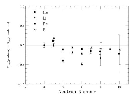
Figure B.1: The difference between the proton density rms radius and the neutron density rms radius obtained from the 790A MeV cross section measurements. Data from [Tan88].
