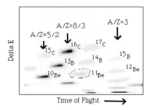
Figure 3.3: A plot of  $\Delta E$  vs. ToF which shows the isotopic separation of fragments that are analyzed in the A1200. The <sup>11</sup>Be beam group is circled.
