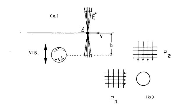
Figure 2.3: [Ber88] As a projectile approaches a target nucleus, the electric field lines are contracted into the plane which is perpendicular to the direction of travel. The resulting electric and magnetic field lines, that can be approximated with two plane waves, Coulomb excite the passing nucleus.
