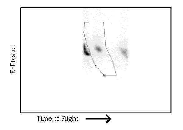
Figure 3.7: The total energy vs. ToF histogram is also used to isolate the <sup>10</sup>Be reaction products. Again, this histogram is gated on the <sup>10</sup>Be reaction products in Figure 3.5.
