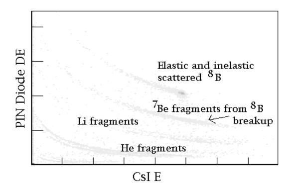
Figure 4.4:  $\Delta E$  vs E showing the <sup>7</sup>Be fragments from <sup>8</sup>B breakup measured in Telescope 2. Li, and He fragments from <sup>8</sup>B breakup are also identified.
