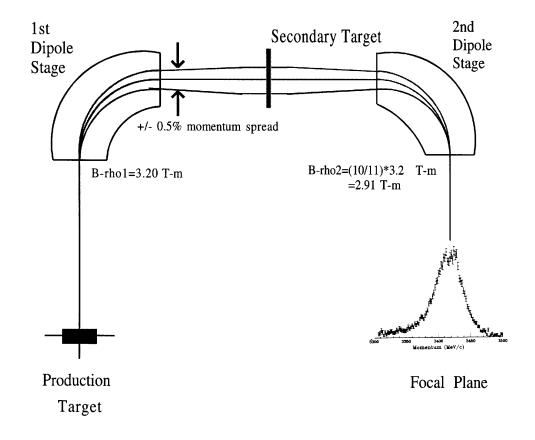
Figure 3.4: The principle of a dispersion matched energy loss spectrometer. A RNB has a momentum spread that is introduced by the production mechanism. However, the optics of the device return the beam to an achromatic focus at the focal plane. The spread in momentum of fragments produced at the secondary target is projected onto the focal plane.
