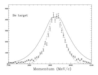
Figure 4.7: The data from breakup in the Be target compared with the predicted  $p_{\parallel}$  distribution of a p-orbital proton bound by 137 keV in a Woods-Saxon potential. The solid(dashed) line represents the distribution without(with) an absorptive cut-off [Bro95a].
