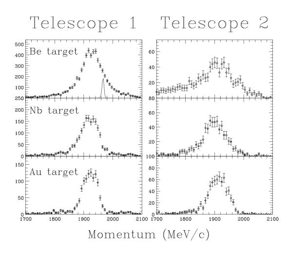
Figure 4.6: The  $p_{\parallel}$  distributions of <sup>7</sup>Be fragments following the breakup of <sup>8</sup>B. The narrow distribution shown with the Telescope 1 Be target data shows the momentum resolution (~0.5%) obtained from one of the energy calibration measurements.
