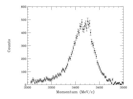
Figure 3.12: The  $p_{\parallel}$  distribution of <sup>10</sup>Be fragments following breakup in the Ta target. The background is low, and the asymmetry hints that a dissipative tail may be present on the low momentum side.
