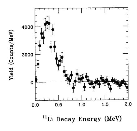
Figure B.3: [Sac93] The decay energy spectrum of <sup>11</sup>Li from Coulomb excitation. A Monte Carlo simulation that accounts for the acceptance of the measurement indicates a peak near 1 MeV in the dipole excitation strength function. The low energy peak is associated with a large separation distance for the <sup>9</sup>Li core and two neutrons that comprise <sup>11</sup>Li
