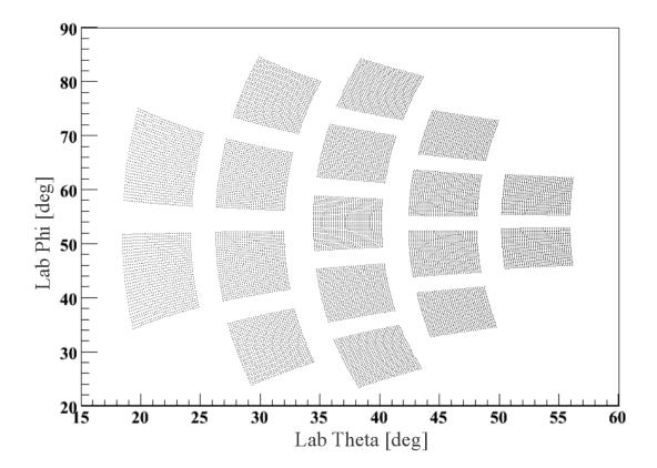
Figure 2.7: Angular coverage of the entire HiRA array.
