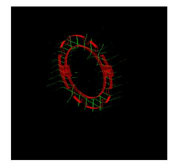
Figure A.4: The red lines are the mechanical drawing of the target frame used to hold a target. The green dots are from the LBAS scans of a target while it was inside the chamber.
