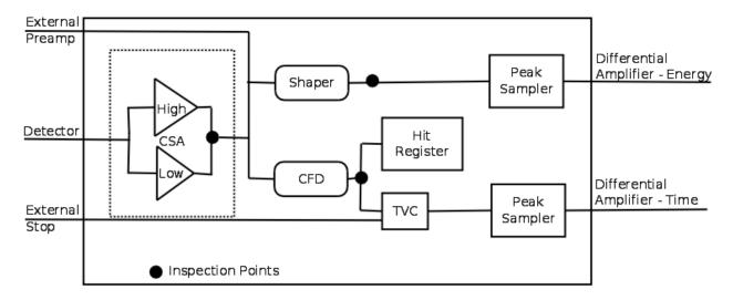
Figure 2.13: Diagram of the ASIC electronics logic. [2,3]
