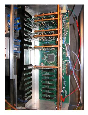
Figure 2.12: Photograph of HiRA motherboard with six chipboards installed.
