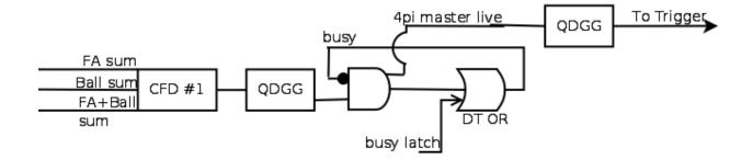
Figure 2.17: Diagram of the  $4\pi$  electronics logic, part(b).
