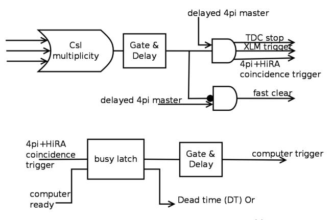
Figure 2.18: Diagram of the coincidence trigger logic. [6]
