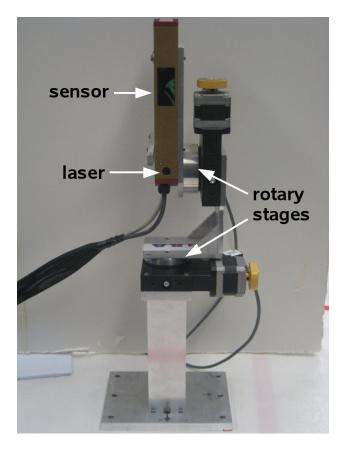
Figure A.2: A photograph of LBAS with components labeled.
