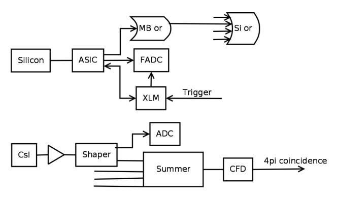
Figure 2.14: Diagram of the HiRA electronics logic. [2,4]
