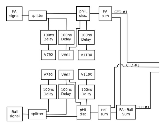
Figure 2.16: Diagram of the  $4\pi$  electronics logic, part (a).
