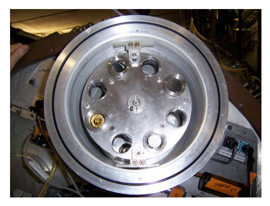
Figure 2.10: Photograph of target carousel which housed all targets used. Pictured, clockwise, are an old scintillator target at 5 o'clock, an old broken gold target at 8 o'clock, and a new empty oblong frame at 11 o'clock.
