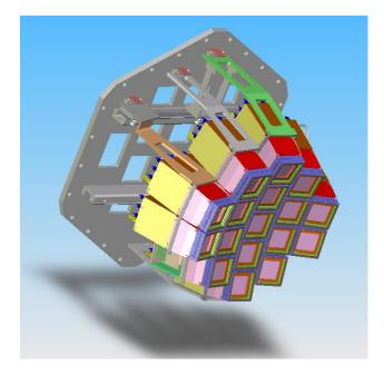
Figure 2.2: Drawing of the HiRA Array mounted on a modified  $4\pi$  flange.
