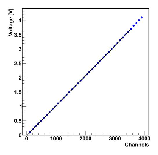
Figure 3.5: A 3rd order polynomial was used to fit the pulser data due to slight non-linearities in the electronics. Shown here are the pulser data and fit for one crystal in telescope 0.
