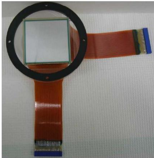
Figure 3.15: HiRA double-sided silicon strip-detector in a circular plastic container.
