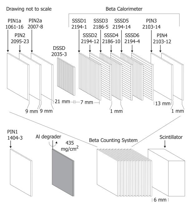
Figure 3.3: Schematic of the  $\beta$  counting system and its position relative to other detectors used during the experiment. Drawing is not to scale and inter-detector distances are given. Silicon detector serial numbers are given below the name of the detector that will be used throughout this document.
