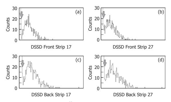
Figure 3.7: Representative DSSD <sup>90</sup>Sr calibration for the front and back of the DSSD. Arrows mark the location of representative software thresholds.
