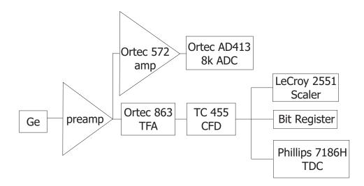
Figure 3.13: Electronics setup for SeGA during experiment NSCL-02004.
