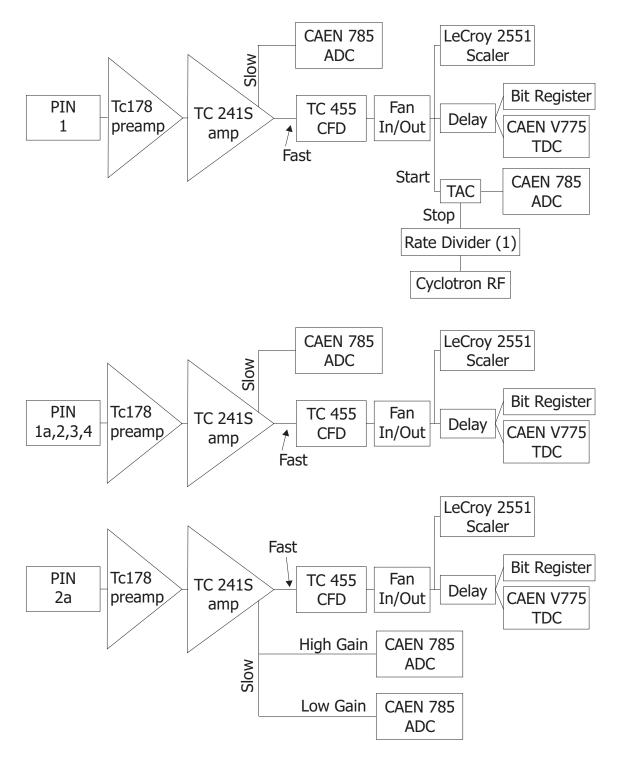
Figure 3.5: Electronics setup for PIN detectors during experiment 02004.
