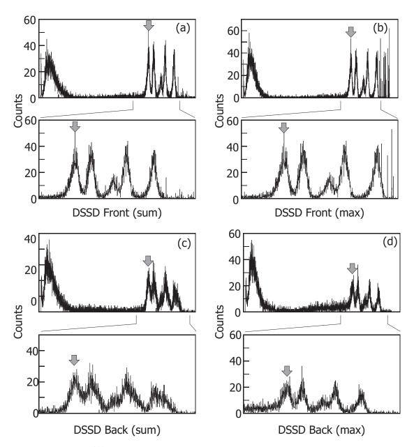
Figure 3.6: DSSD  $^{228}$ Th calibration for the front and back of the DSSD. Arrows mark the 5.4 MeV  $^{228}$ Th alpha peak that was used for gain-matching. Panels a,c report the total energy collected in the DSSD determined from the sum of the energy deposited in each strip. Panels b,d report the maximum energy collected in one channel.
