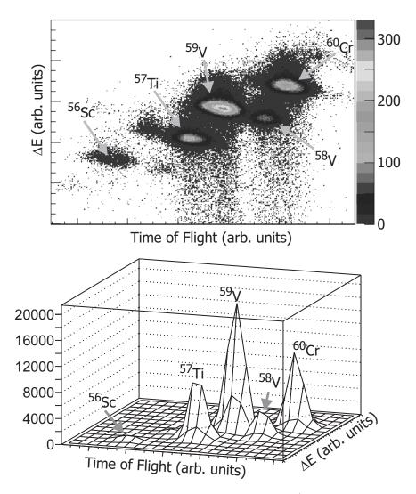
Figure 3.2: Particle identification using Time of Flight (start from scintillator 2 m upstream of the DSSD and stop from the cyclotron rf signal) and energy loss in the first PIN detector. <sup>56</sup>Sc is well separated from the other implanted isotopes even though it constitutes <1% of the total beam.
