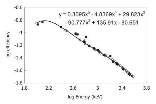
Figure 3.19: Efficiency of the array of 12 HPGe detectors as a function of energy. The diamonds represent calculations with the MCNP code using a point source geometry at the DSSD location. The squares represent experimentally determined efficiencies. A fifth order polynomial relating the energy with efficiency is shown by the solid line.
