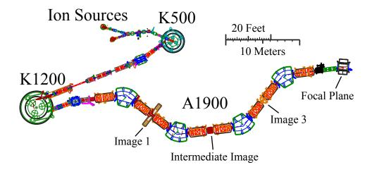
Figure 4.1: Schematic depicting NSCL ion sources, K500 and K1200 cyclotrons, and A1900 fragment separator. The production target is located in the blue box after the exit of the K1200 cyclotron and the before the entrance of the A1900 fragment separator.
