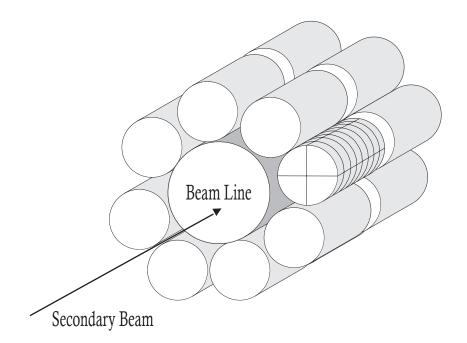
Figure 4.5: Cartoon of Barrel SeGA configuration. Figure modified from Ref. [96].
