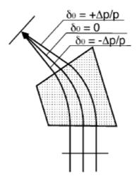
Figure 4.3: Cartoon depiction of lateral dispersion-matching, taken from Ref. [92]. Dispersion of rays with different momenta is compensated by the dispersion of the spectrometer.
