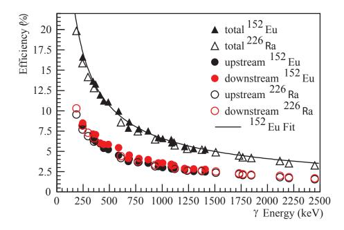
Figure 5.4: Efficiency curves for  $^{152}$ Eu and  $^{226}$ Ra calibration source measurements.
