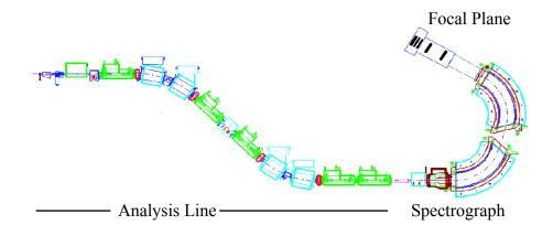
Figure 4.2: Schematic depicting analysis line and spectrograph components of S800 Spectrograph.
