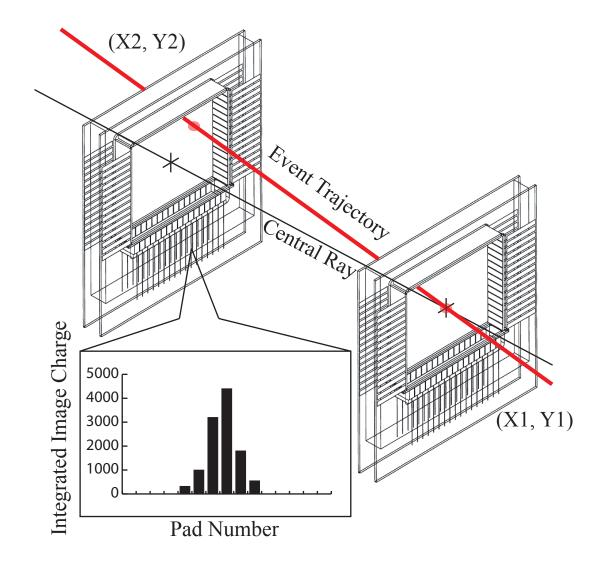
Figure 4.4: Layout of CRDC detectors and cartoon of cathode position determination. Figure taken originally from Ref. [93], modified by Wes Hitt in Ref. [94].
