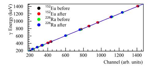
Figure 5.3: Channel-Energy relationship and fits for  $^{152}$ Eu and  $^{226}$ Ra calibrations, taken before and after the experiment.
