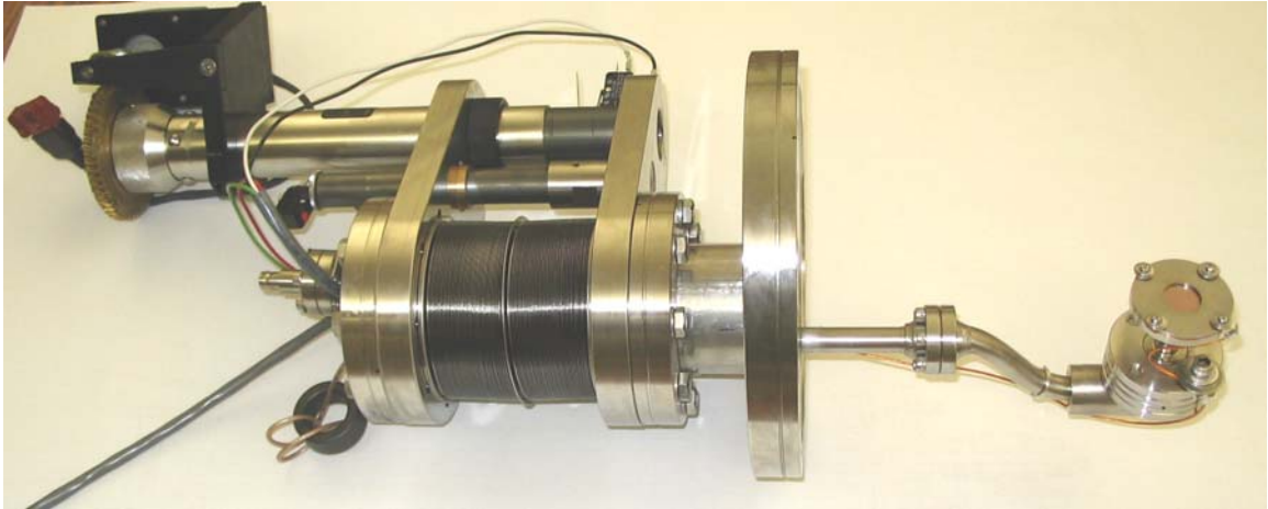
Figure 31: Picture of the movable fast Faraday cup used to measure longitudinal beam profiles.
