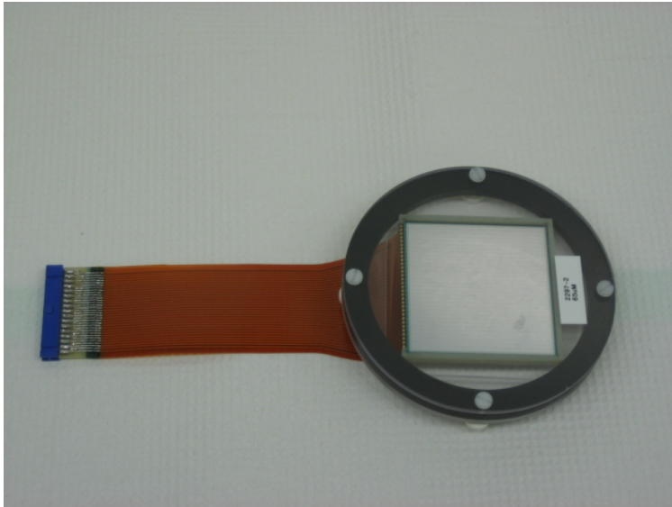
Figure 3.14: Photograph of a HiRA single-sided silicon strip-detector ( \Delta E ) in a circular plastic container. The brown band extending outside the container is the signal cable.
