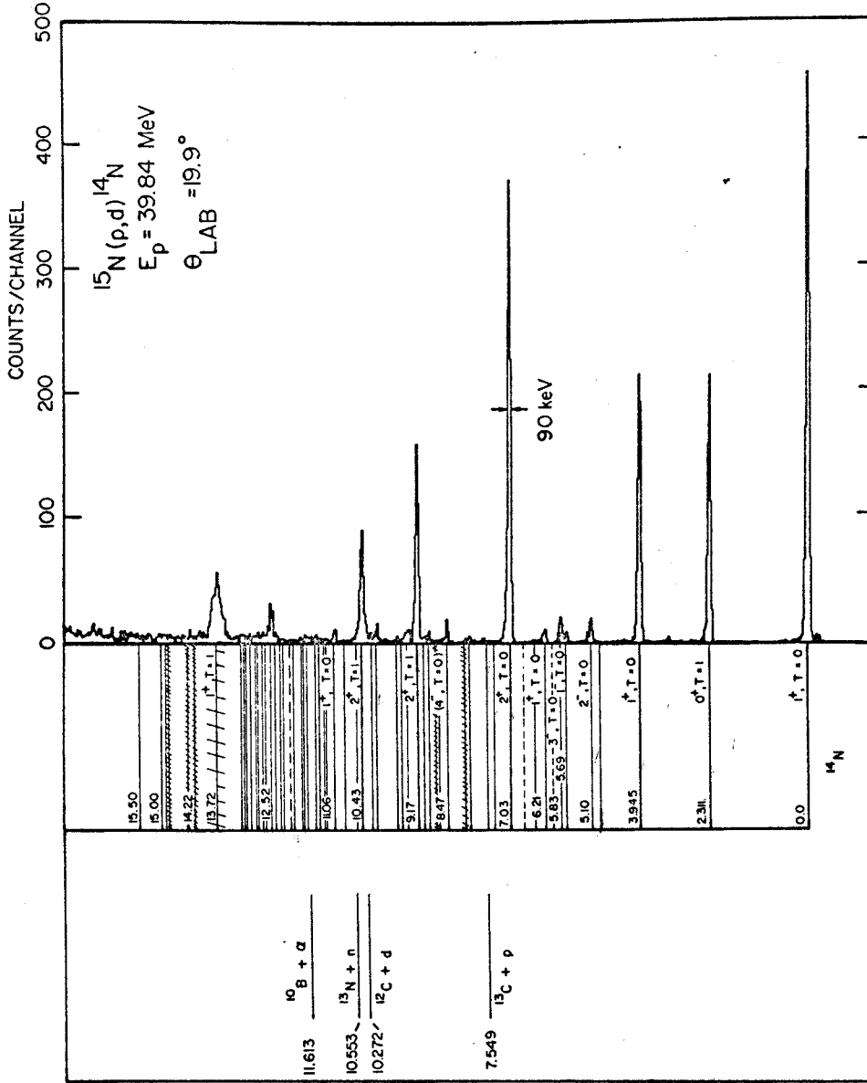
Figure V-15.: Energy level diagram of ^{14}\text{N} displayed beside a deuteron energy spectrum from the ^{15}\text{N}(p,d)^{14}\text{N} reaction for E_p=39.84 \text{ MeV} and \theta_{\text{LAB}}=19.9^\circ . The seven strong levels are formed by 1p neutron pickup.
