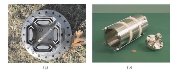
Figure 3.2: Examples of component of the LEBIT beam transport system. (a) 90 degree quadrupole deflector; (b) Einzel lens.
