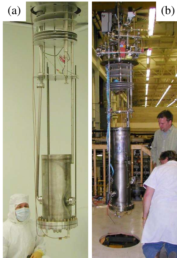
Figure 5. Photographs of (a) \beta_m = 0.16 QWR and (b) \beta_m = 0.085 QWR on the RF test stand.
