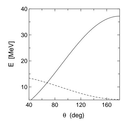
FIG. 2: Kinematics of the <sup>4</sup>n-proton scattering in the laboratory. The solid line shows the proton recoil energies in the interval  $E_p = 21$  - 38 MeV, for scattering angles between 95 - 180 degrees. The dashed line is the respective <sup>4</sup>n energy (per nucleon).
