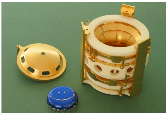
Fig. 4. The LEBIT high-precision Penning trap with the endcap electrode removed.
