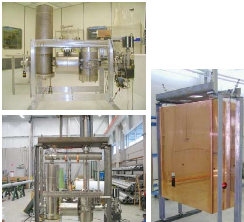
Figure 5.51: Photographs of components for the prototype cryomodule. Top left: cold mass in the clean room. Bottom left: module in assembly area. Right: test fit of the nitrogen shield to top plate.
