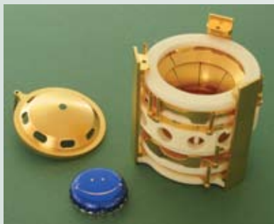
Figure B: The electrodes from the 9.4 Tesla Penning-trap mass spectrometer at the LEBIT facility at the NSCL.
