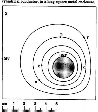
10. The figure shows the equipotential surfaces for a long cylindrical conductor, in a long square metal enclosure.
