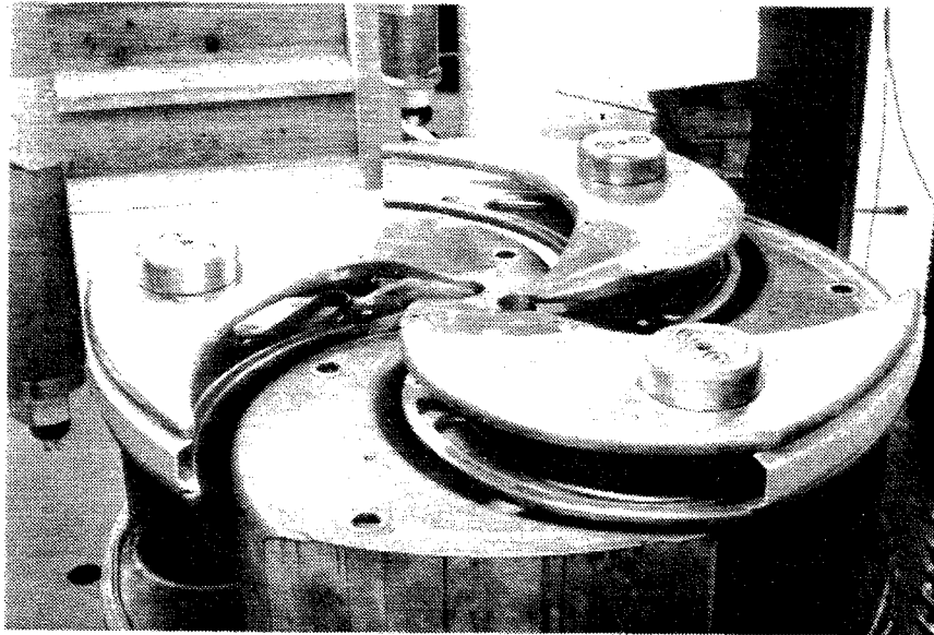
Figure 15. -- Photo showing the accelerating electrode structure mounted on the lower magnet pole. The inter-connection of the electrodes shows at the center.
