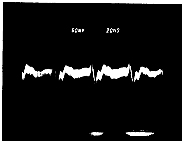
Fig. 2.--Typical signal from the phase-probe for a beam current of 0.6 A.
