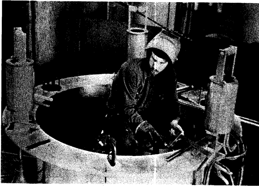
FIG. 15. Aluminum heat shield to be installed between 4° K superconducting coil and outer room temperature wall. It will run at liquid nitrogen temperature.
