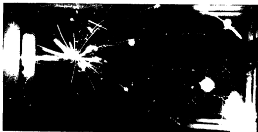
Collision of an argon nucleus with a lead nucleus at an incident energy of 72,000 MeV in a streamer chamber. The nucleus is incident from the left. (From L. S. Schroeder, Streamer chambers—their use for nuclear science experiments , Nucl. Instr. Meth. , 162:395-404, 1979)
