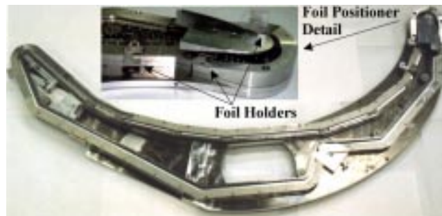
Figure 5. K1200 stripping foil mechanism.
