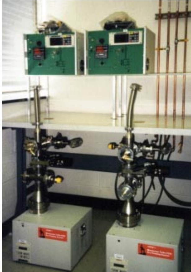
Fig. 1: The Gamma Annealing Station showing the vacuum systems (below) and the controller boxes (above).
