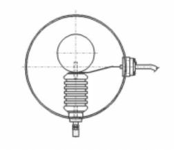
Above is a cross section through the resistor tank, showing one of the insulating posts and spheres. The resistors are connected between the four spheres.
