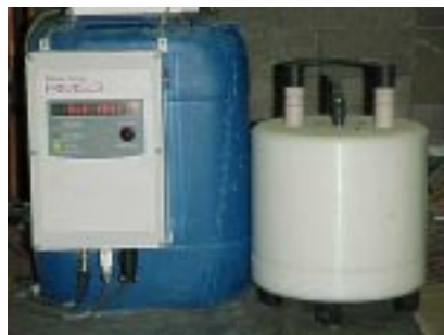
Figure 4: A neutron area monitor by Eberline Corp. is shown. The detector, model SWENDI-II, is shown on the right. The control unit is Eberline's model RMS-3.
