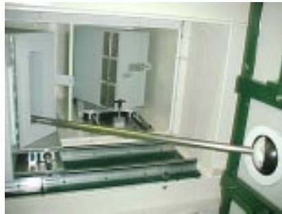
Figure 8: A remote handling tool allows one to remove an activated target from the A1900 production target chamber and to place it into a storage box.
