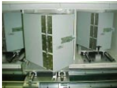
Figure 9: Three lead-shield target storage boxes are shown.
