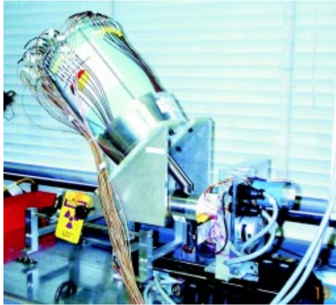
Figure 2: Segmented germanium detector mounted in the test stand.
