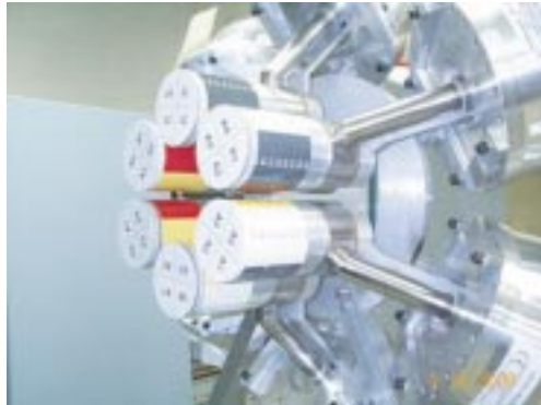
Figure 1: Photograph of the germanium array configuration that was used in the Xe Coulomb excitation experiments.
