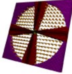
Figure 2: The 57.5 MHz 4-vane RFQ with the characteristic magnetic field of the TE_{21(0)} mode.
