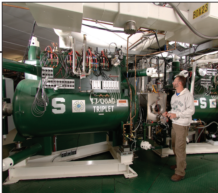
One of eight superconducting quadrupole triplets that are used to focus the beam in the A1900 fragment separator.
