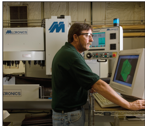
CNC programming of a lathe with live tooling.
