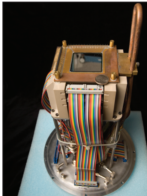
The Beta Counting System detector stack. The detector in view is the DSSD implantation detector.
