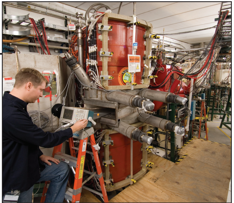
The picture shows the front face of the iron blocks of the sweeper magnet placed above and below the vacuum chamber for the charged particles that are deflected by the magnet. A graduate student is adjusting signals from a detector inside the focal plane detector box.
