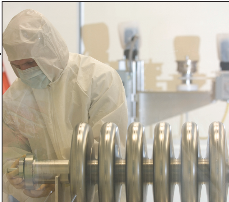
A superconducting radiofrequency cavity made from niobium is being assembled in preparation for testing.
