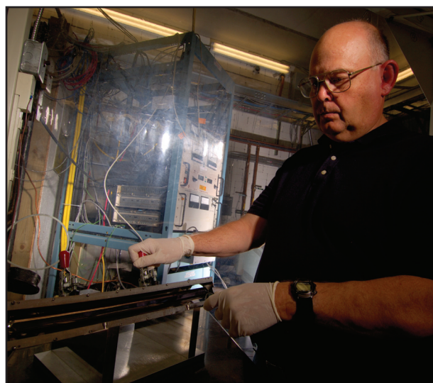
On the bench is a deflector for the K1200 cyclotron, called the E2 deflector. The septum is removed and one can see the high voltage electrode.
