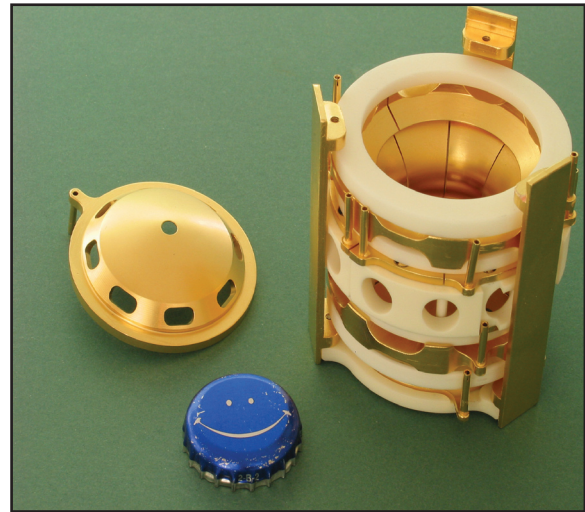
The high-precision and gold-plated electrode system of the LEBIT Penning trap which is located inside the large 9.4 Tesla magnet system of LEBIT. The ions are captured inside this trap and their mass is measured here
