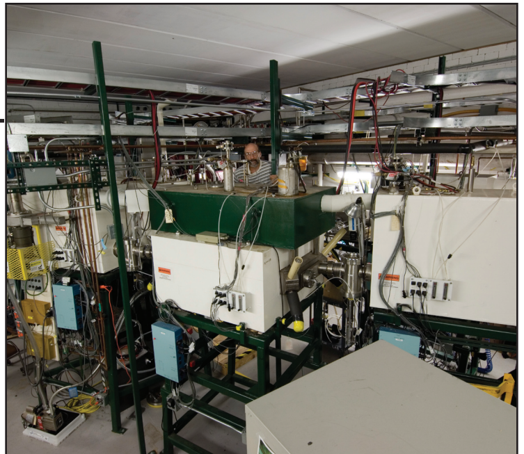
Some of the superconducting magnets that deliver beam to the experiments in the N4 vault.
