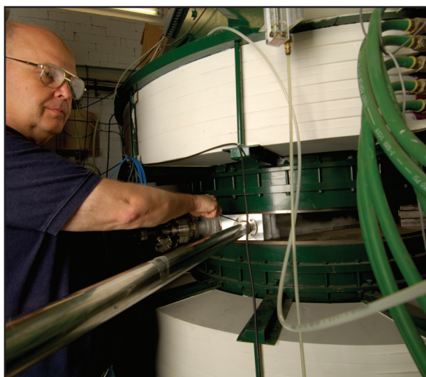
The Deflector Test Stand. It is placed inside a magnetic field. The long tube at the bottom of the picture is the high voltage feedthrough.
