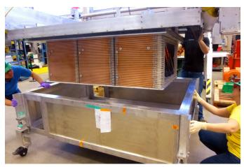
The detector portion of the SAMURAI TPC is being lowered into a large aluminum enclosure, which provides protection and insulation. The TPC is now ready for testing and debugging, which will begin next week.
