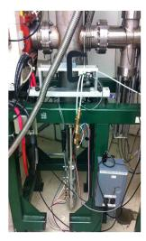
A prototype Halo Scraper Ring (HSR) is installed in the coupling line between the K500 and K1200 cyclotrons. It is being tested for its ability to detect beam loss and shut the beam off to prevent damage to components.
