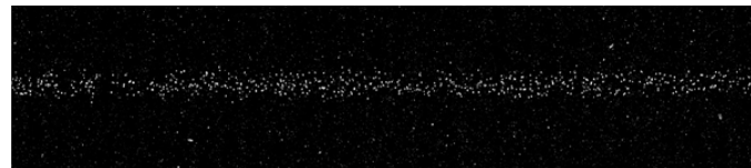
Typical image of the EBIT electron beam taken with an X-ray pinhole camera. Each white dot is the result of an X-ray hitting a pixel of the CCD.
