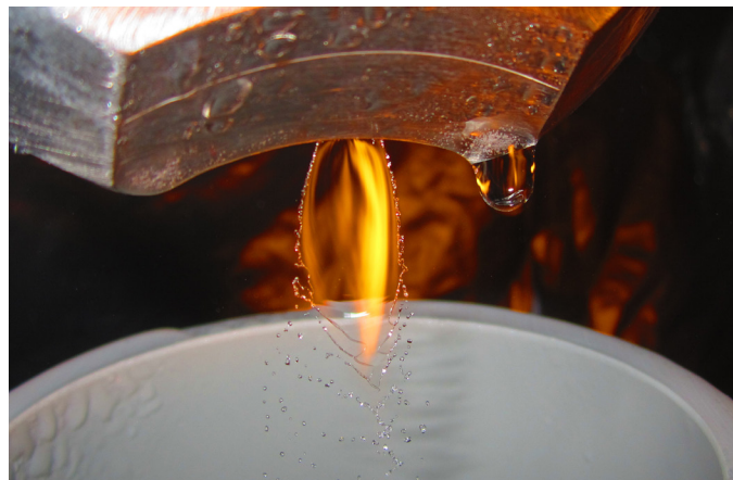
A water jet thin film is measured as part of development of the FRIB liquid lithium stripper. The water drop at right can help give an indication of scale.
