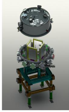
Mechanical design rendering of the CFFD. The 4 PPACs are shown (yellow frames) surrounding the target in the center of the chamber. The beam will enter from the left and pass through the position sensitive MCP before impinging on the target.
