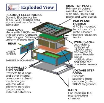
The picture shows a schematic drawing of  $S\pi RIT$ . One can explore various parts of the TPC interactively on the website .
