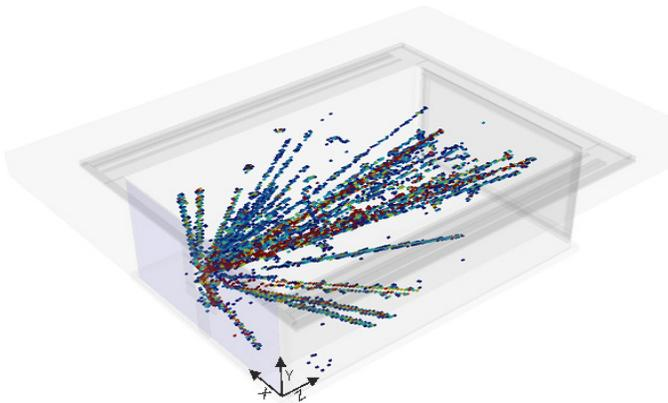
The figure shows the ionization in the TPC for event. The beam initially travels in the Z direction and strikes a target located approximately 1 cm upstream of the TPC.
